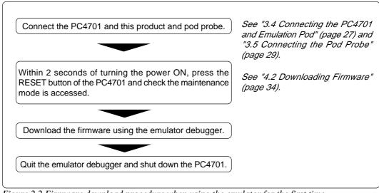
Figure 2.2 Firmware download procedure when using the emulator for the first time
